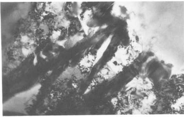
Figure 23 Very complex transformation to mixture of carbides and intermetallic phases, accompanied by intense strain bands. BW 19, aged at 700° C, \times 53 280.
