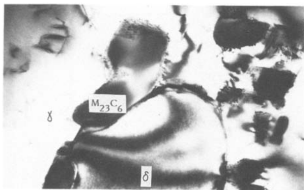
Figure 12 Strain fields accompanying transformation to M 23 C 6 carbides at δ/γ boundaries. BW 15, aged at 850° C, × 53 280.
