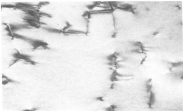
Figure 18 Very limited matrix precipitation in austenite after creep testing at 600°C. BW 15, aged at 850°C, \times 69\,930 .
