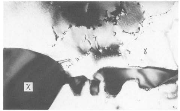
Figure 26 Partial spheroidisation of transformed intermetallic \chi -phase following ageing at 850° C. BW 19, aged at 850° C, \times 35 298.
