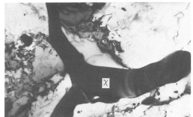
Figure 29 Complete transformation of original \delta -ferrite laths to intermetallic \chi -phase following creep testing at 600° C. BW 19, aged at 700° C, \times 13 320.
